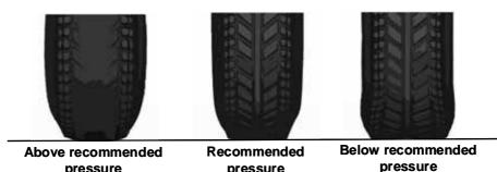
Figure 2.1 Diagrams showing effects of over and under-inflated tyres (courtesy of Michelin UK)
