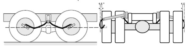
Figure 3.7 Schematic diagrams of a TPCS air hose arrangements on a tractor unit (TPC International)
