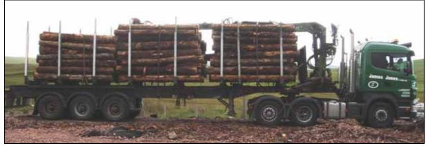
Figure 4.2 Photograph of the loaded James Jones TPCS 6x2 TAG unit with super single tri-axle trailer during hauling operation on the A897 public Road, July 2007
