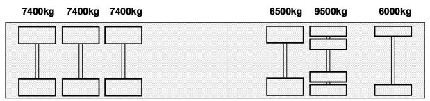
Figure 4.3 Schematic of James Jones TPCS 6x2 TAG unit with super single tri-axle trailer
