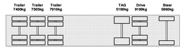
Figure 3.2 Schematic of underside of the loaded test vehicle showing the measured axle loads in kg
