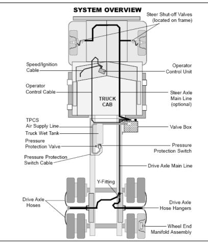
Figure 3.6 Schematic diagram of a TPC system on a tractor unit (TPC International)
