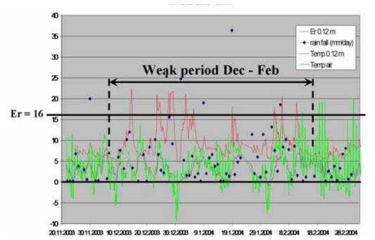
Figure 1.5 Output screen from a Percostation on the B871 showing basecourse dielectric value & temperature, air temperature and daily rainfall. The weak period for timber traffic is based on a basecourse dielectric value of 16.
