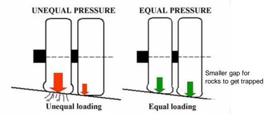
Figure 2.3 Effect of equal pressure in twin tyres on a crowned road (TPC International)
