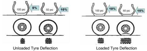
Figure 2.4 Effect of lowered tyre pressures on tyre sidewalls (TPC International)
