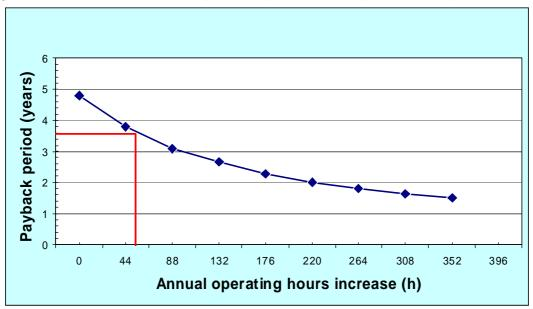
Figure 4.1 Payback years v. Annual operating hours increase for the Highland test vehicle, medium duty working (10%-30% off highway), no improvement in fuel consumption assumed
