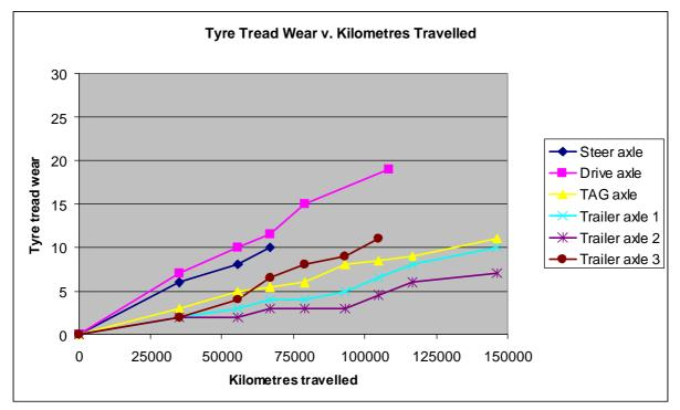
Figure 4.4 Graph of tyre tread wear v. distance travelled by test vehicle
