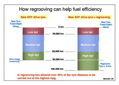
Figure 5.1 Diagram showing how regrooving of a tyre can help fuel efficiency
